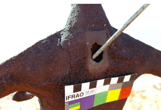
Figure 3 Salt crystals on the lower legs and pin point corrosion
